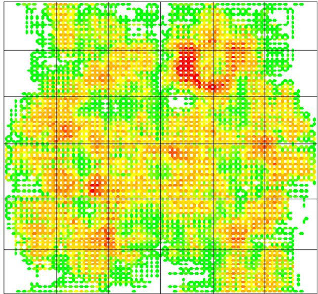
Fig. 14. A typical global routing congestion map. Each edge corresponds to approximately 100 global routing edges (and to approximately 10000 detailed routing channels). Red, orange, yellow, green, and white edges correspond to an average load of approximately 90–100%, 70–90%, 60–70%, 40–60%, and less than 40%.
