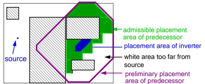
Fig. 11. Computation of the feasible area for a predecessor of an inverter. From all points that are not too far away from the placement area of the inverter (blue) we subtract unusable areas (e.g., those blocked by macros) and points that are too far away from the source. The result (green) can again be represented as a union of octagons.
