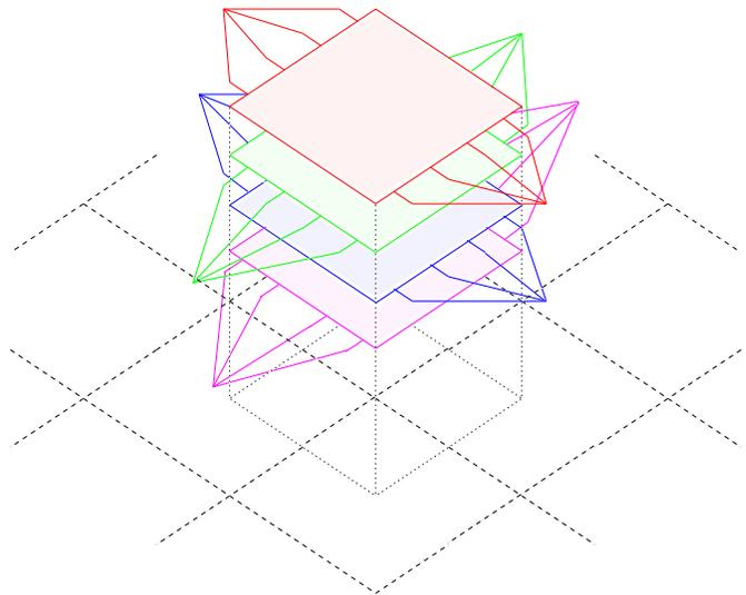
Fig. 13. An instance of the edge-disjoint paths problem for estimating global routing capacities. Dashed lines bound global routing regions. Here we show four wiring planes, each with a commodity (shown in different colors), in alternating preference directions.
