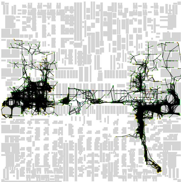
Fig. 12. Gigahertz clock tree built by BonnClock based on the result of BonnCycleOpt shown in Figure 9. Colors indicate different arrival times as in Figure 10. Each net is represented by a star connecting the source to all sinks.
