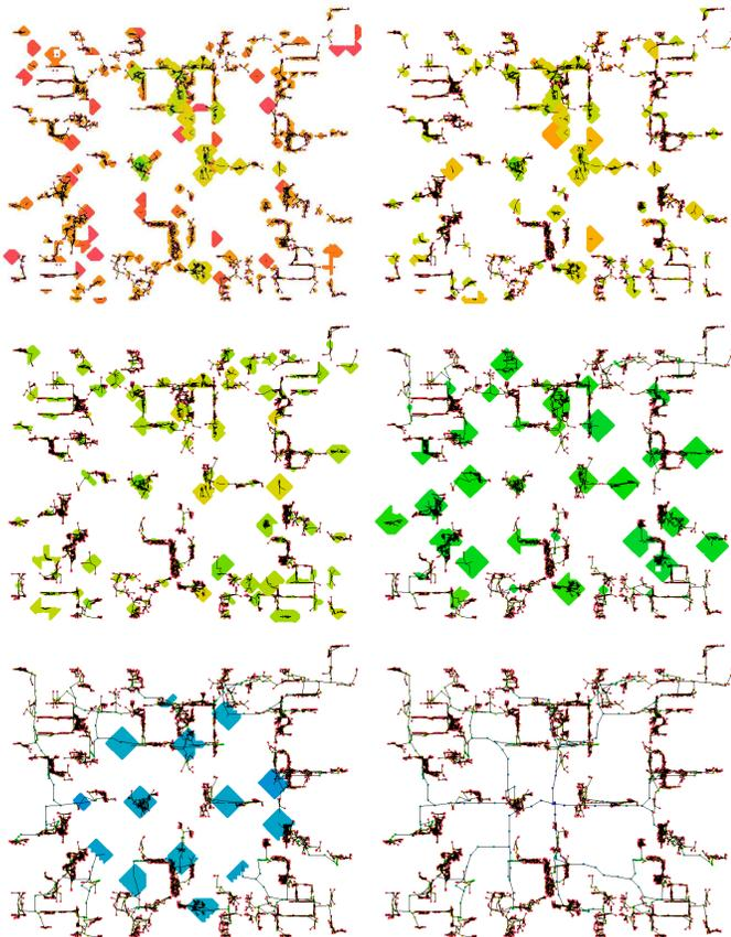
Fig. 10. Different stages of a clock tree construction using BonnClock. The colored octagons indicate areas in which inverters (current sinks) can be placed. The colors correspond to arrival times within the clock tree: blue for signals close to the source, and green, yellow, and red for later arrival times. During the bottom-up construction the octagons slowly converge to the source, here located approximately at the center of the chip.
