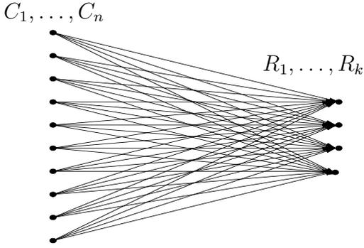
Fig. 2. Modeling multisection as a Hitchcock transportation problem. All arcs are oriented from left to right and are uncapacitated. Vertices on the left correspond to movable objects and have supply  $a_1, \dots, a_n$ . Vertices on the right correspond to subregions and have demand  $b_1, \dots, b_k$ . The cost of an arc  $(C_i, R_j)$  is  $d(i, j)$ . Note that  $k \ll n$ .
