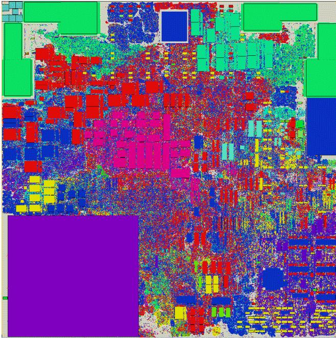
Fig. 16. A system on a chip designed in 2006 with BonnTools. This 90nm design for a forthcoming IBM server has almost 5 million nets on the top level and runs with frequencies up to 1.5GHz.
