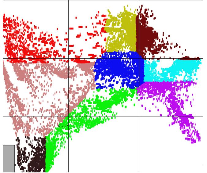
Fig. 3. Example for multisection: objects are assigned to  $3 \times 3$  subregions. The colors reflect the assignment: the red objects are assigned to the top left region, the yellow ones to the top middle region, and so on. This assignment is optimal with respect to total  $\ell_1$ -distance.
