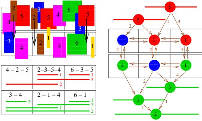
Fig. 4. An example with two zones and six regions, each of width 10 (top left), the supply (red) and demand (green) regions and intervals with their supply and demand (bottom left), and the minimum cost flow instance (right) with a solution shown in brown numbers. To realize this flow, objects of size 2, 2, and 5, respectively, have to be moved from the top regions downwards.
