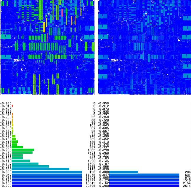
Fig. 9. Slack histograms showing the improvement due to clock skew scheduling and appropriate clock tree synthesis; left: zero skew, right: with BonnClock trees. Each histogram row represents a slack interval (in ns) and shows the number of slacks in this range. The placements on top are also colored according to these slacks.
