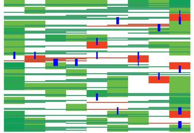
Fig. 5. Small part of a real chip in legalization. Supply regions and intervals are shown in red, demand regions and intervals in green. The blue edges represent the minimum cost flow, and their width is proportional to the amount of flow.
