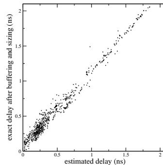
Fig. 6. The simple timing model used for topology generation matches actual timing results after buffering well.
