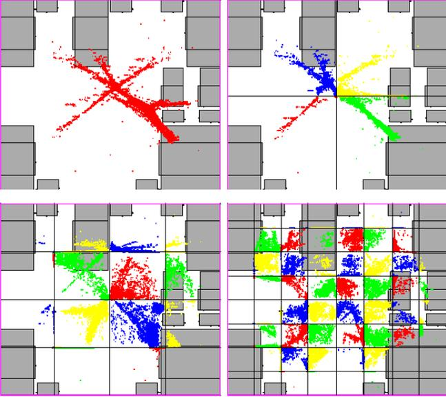
Fig. 1. The initial four levels of the global placement with 1, 4, 16, and 64 regions. Colors indicate the assignment of the movable objects to the regions.
