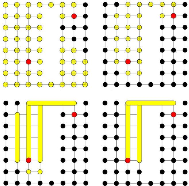
Fig. 15. Dijkstra’s algorithm without (left) and with (right) future cost, point-based (top) and interval-based (bottom). We require a shortest path from the red vertex in the bottom left to the red vertex in the upper right part. Points or intervals labeled by Dijkstra’s algorithm are shown in yellow. The running time is roughly proportional to the number of labeled points (50 versus 24) or intervals (7 versus 4 in this example).
