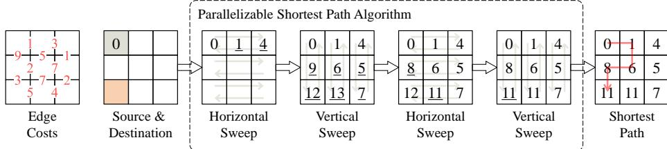
Figure 4: Shortest Path via Alternating Sweeps.
