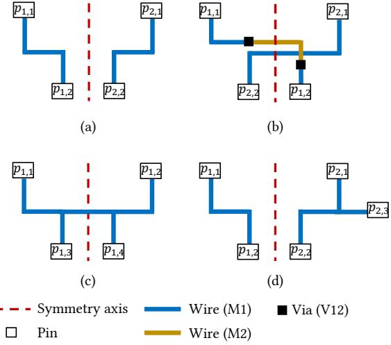
**Figure 6: Examples of symmetry constraint variants:** (a) Mirror-symmetry. (b) Cross-symmetry. (c) Self-symmetry. (d) Partial-symmetry [12].
