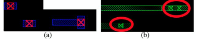
**Figure 2:** (a) Two most-left vias are horizontal vias, and the one on the right side is a vertical via. (b) Double cut via insertion compared to single cut.
