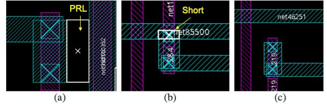
**Figure 3:** Double cut via insertion with (a) a parallel run length (PRL) violation; (b) with short violation and (c) a well inserted via without violations.
